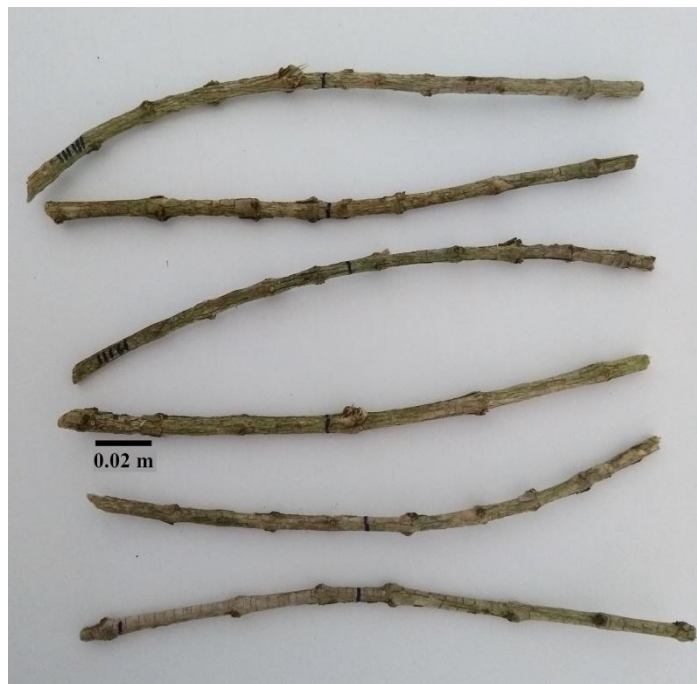
Figure 3 - Specimens produced from the branches of a coffee plant sample and subjected to tensile tests, in a universal testing machine, in the direction parallel to the fibers.
