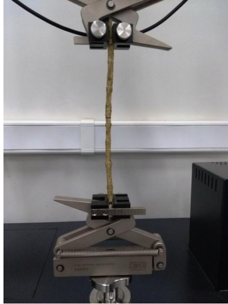
Figure 7 - Specimen produced from the branch of a coffee plant sample being subjected to tensile testing, in a universal testing machine, in parallel direction to the fibers.
