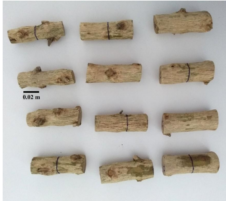
Figure 1 - Specimens produced from the trunks of a coffee plant sample and which were subjected to compression tests in the universal testing machine, in parallel and perpendicular to the fibers.
