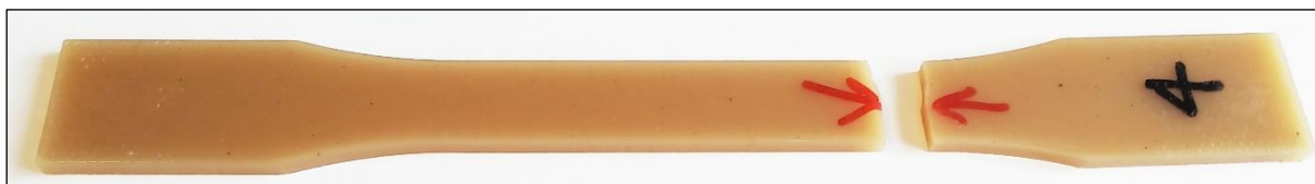
Figure 12 Picture of the rupture of a composite specimen PLANFC40 6 during the tensile test.
