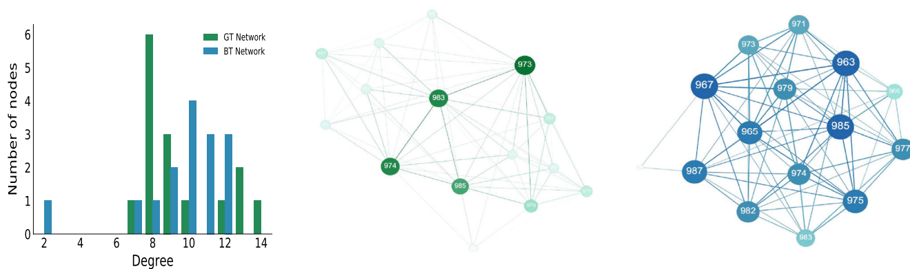
Fig. 7 Degree distribution comparison of ClassA GT (green) and BT (blue) undirected networks, followed by the topologies of the GT and BT networks. The networks are visualized with different node sizes depending on their degree centrality values, bigger node size implies higher centrality
