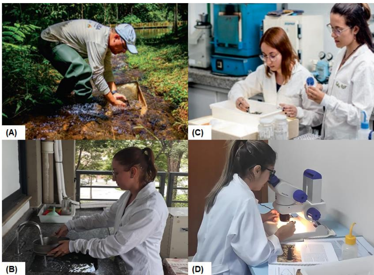
Figure 4: Sample processing and larvae identification. A) Sampling with kick-net collector downstream; B) Sediment washing over sieves at laboratory; C) Sorting on trays over a lightbox; D) Identifying larvae.
