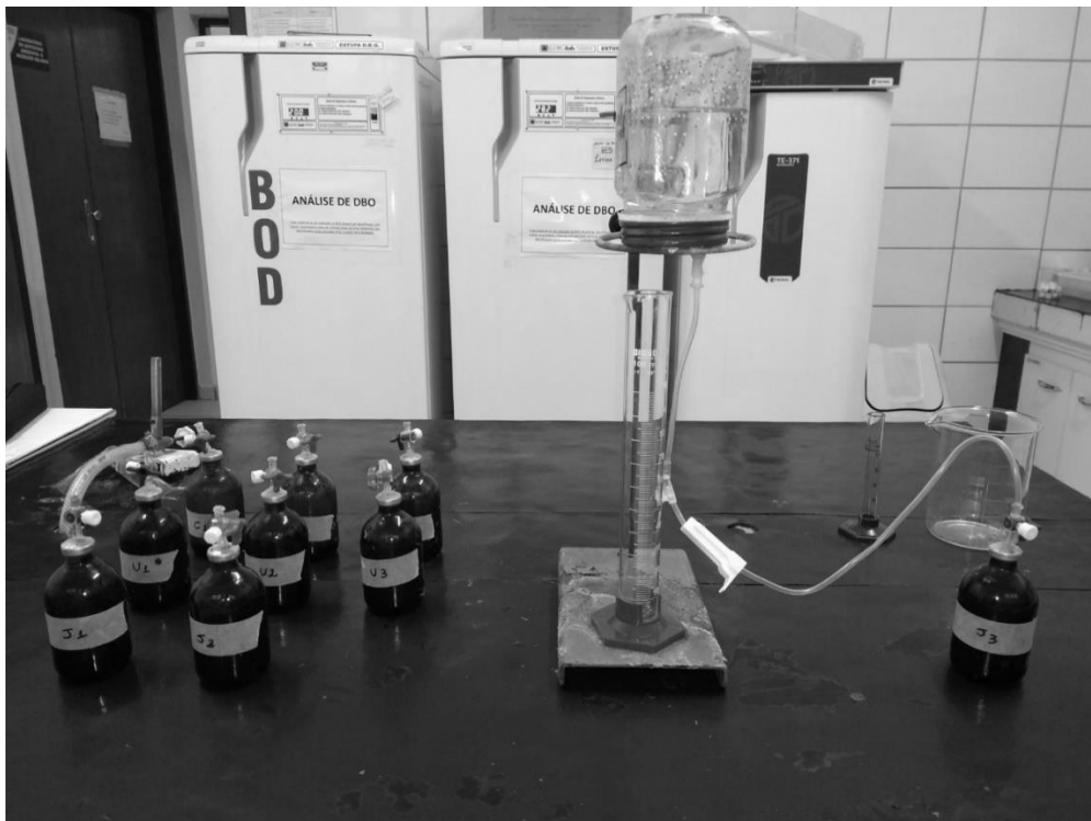
Figure 1 – Experimental apparatus used for measuring the CH 4 volume produced inside the reactor flasks.
