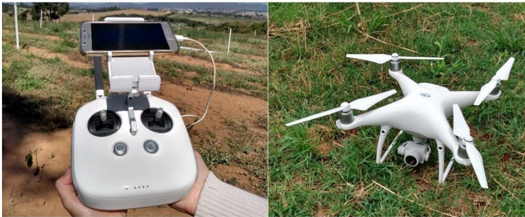
Figure 4. Equipment used for image collection. Remotely piloted aircraft (RPA), a quadcopter type.
