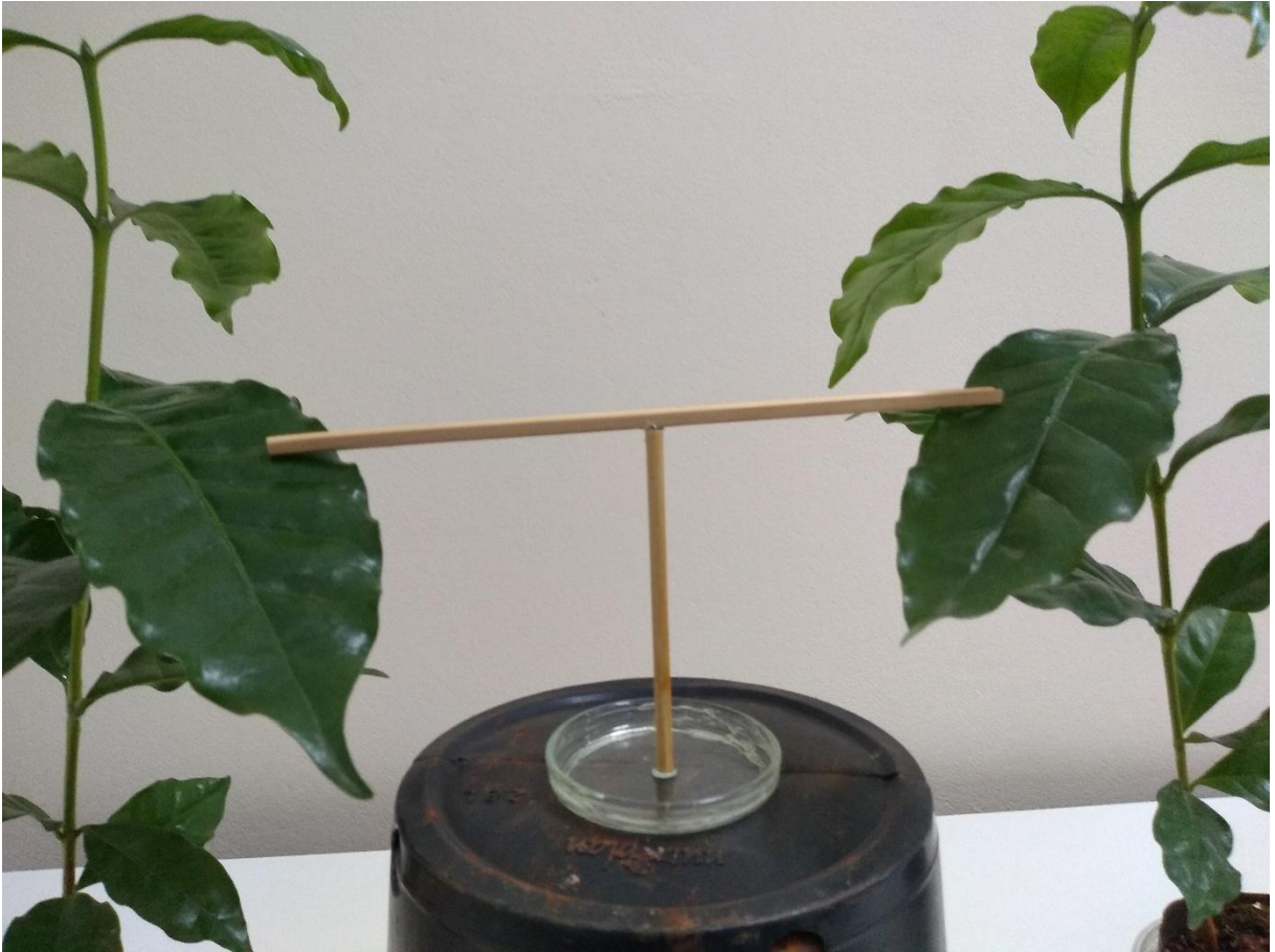
Figure S1- Arena used to test the preference of the southern red mite ( Oligonychus ilicis ) between conspecific-infested and uninfested coffee plants. A wooden T-shaped stick (18 cm width, 9 cm height) attached to the center of a Petri dish bottom (5 cm diameter).
