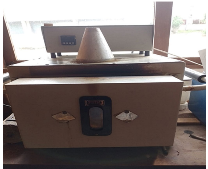
Figure 1: The Jung® muffle furnace used for the production of poultry litter biochar through the pyrolysis process.
