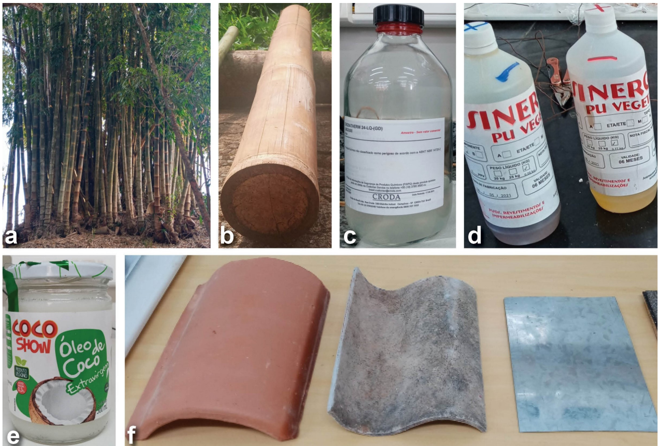
Figure 2: Materials: Dendrocalamus giganteus clump where the research material was harvested (a), piece of bamboo culm as the used (b), commercial CrodaTherm 24 PCM (c), (d) resin used for sealing, PU vegetal – type "V" commercial. Commercial coconut oil (e) and used specimens of building materials (f) respectively from left to right: ceramic tiles, fiber cement, and metal sheet.
