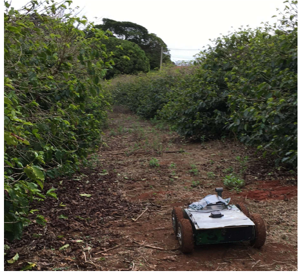
Figure 1 Rover equipped with u-blox C102-F9R application board and antenna ANN-MB-01 (black box in the gray area over the robot's roof) used in the experimental test.
