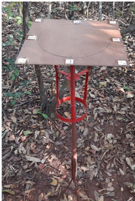
Supplementary Figure 3. Anemometer built to measure wind speed and wind direction inside the study area. Cerradão fragment, UNESP Farm, Selvíria, state of Mato Grosso do Sul, Brazil.
