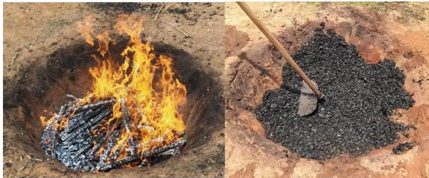
Figure 2S: Trench during and after the pyrolysis process to produce coffee wood biochar.
