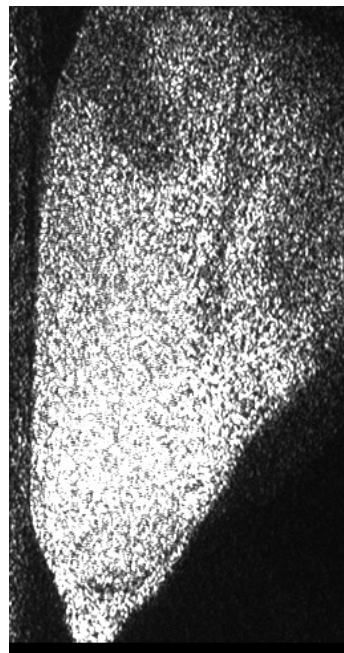
Figure 1.3: First image of a maize seed illuminated by a HeNe laser beam.
