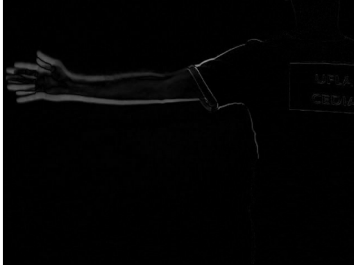
Figure 1.17: Subtraction of two consecutive images of a person moving his arm. Reprinted from Optics and Lasers in Engineering, 50, 3, R. P. Godinho, M. M. Silva, J. R. Nozela, R. A. Braga, On-line biospeckle assessment without loss of definition and resolution by motion history image, Pages 366-372, Copyright (2012), with permission from Elsevier.
