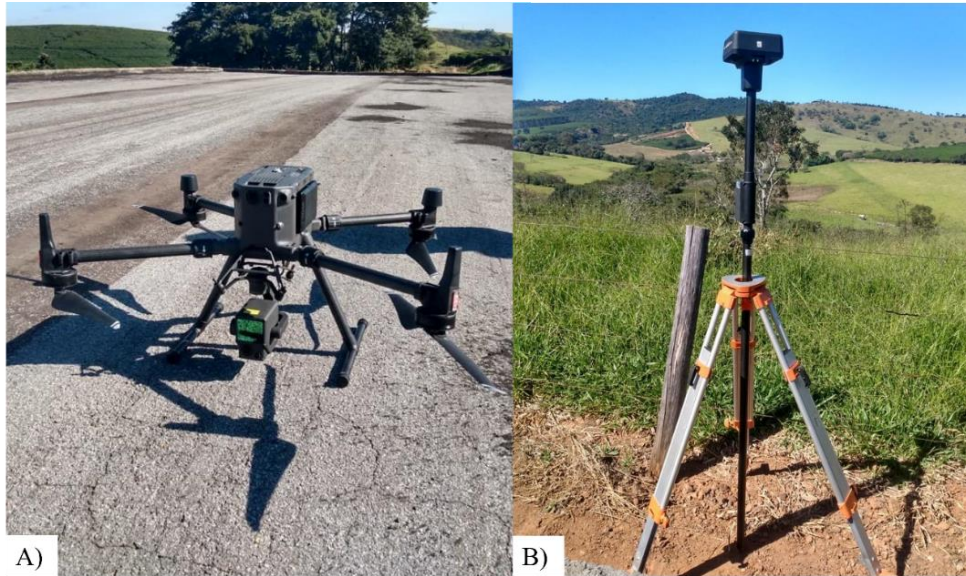
Figure 2. A) Matrix 300 RTK with Zenmuse L1 coupled; B) DRTK-2 base fixed to the ground.
